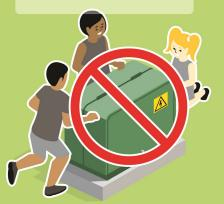
Keep areas surrounding the padmounted transformer clear so that workers can safely maintain transformers as needed. Keep shrubs and structures at least 10 feet away from the transformer doors and 4 feet away from the sides.
